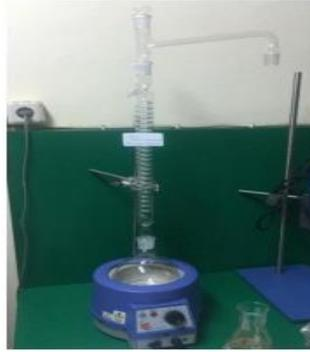
**Gambar 2. 6 Proses Refluks (Hidayat *et al.*, 2019)**
