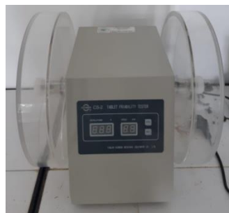
Gambar 12. Friabilator tester (guoming)
