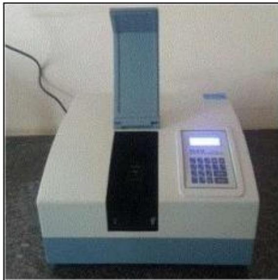
Gambar 2.6 Spektrometer UV-Vis (single beam) (Sumber:Karnakar, 2020)
