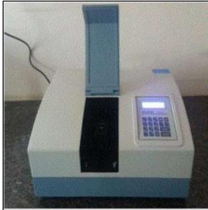
Gambar 2.4 Spektrometer UV-Vis (single beam) (Karnakar *et al.*, 2020).
