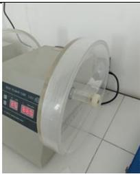
A tablet friability tester. It is a white machine with a large, clear plastic drum. The machine is used to test the mechanical strength of tablets by tumbling them.                  |
